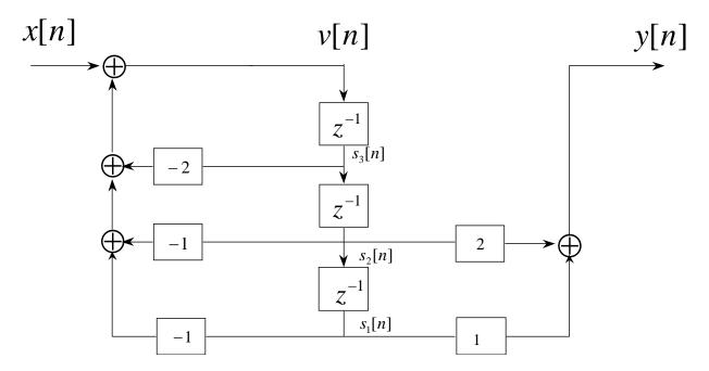
From the diagram we can determine the state space equations as
