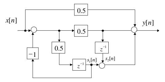
Determine the State Space equations and the Transfer Function.
