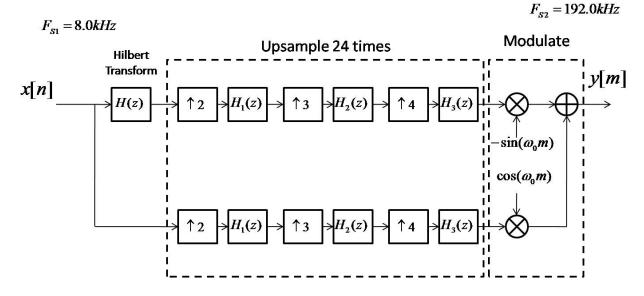
The signal to be modulated has a bandwidth B = 3.5kHz, it is sampled at  $F_{s1} = 8.0kHz$  and we want to SSB modulate it to a carrier with frequency  $F_0 = 80.0kHz$ . In order to do this, we upsample the signal by 24 times in three stages as shown. Design each filter as equiriplle (using *firpm*) with an attenuation of 40dB in the stopband.
