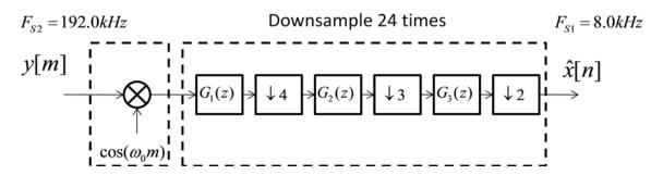
Downsampling the signal 24 times is performed in three stages as shown. Design the three filters again as equripple, with 40dB attenuation in the stopband.
