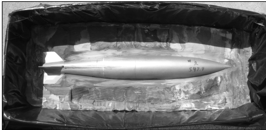
Figure 8. Prototype in Mold Box Prior to Adding Mold Rubber Compound
