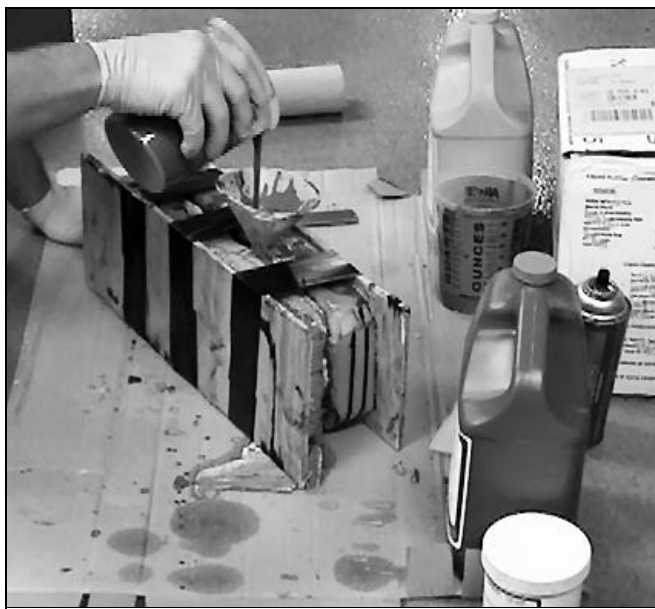
Figure 10. Pouring the Resin Mixture into the Model Mold
