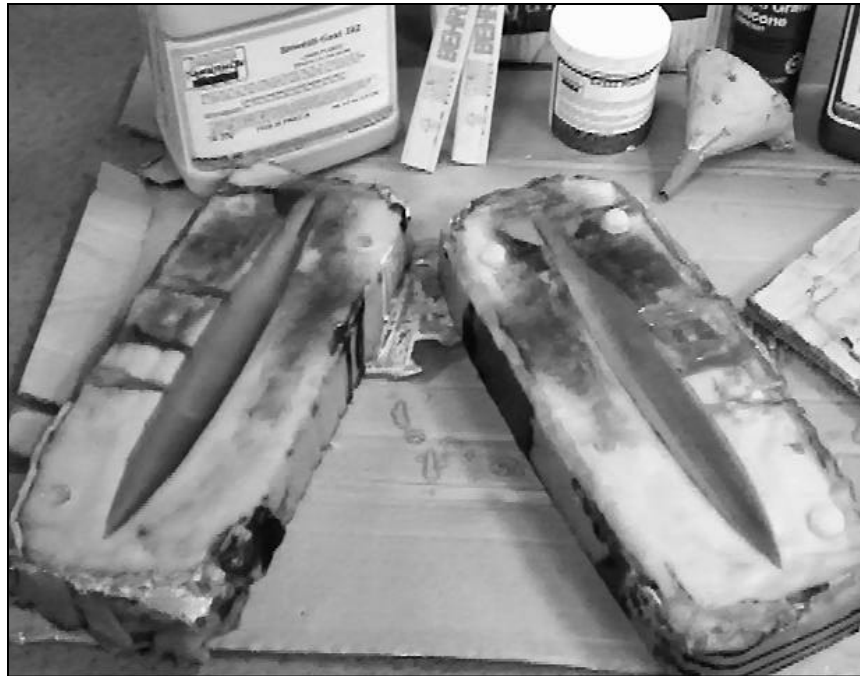
Figure 9. Finished Rubber MK-84 Model Mold
