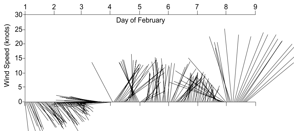
Figure 4. Hourly wind speed and direction during February 2001 as measured at 57.08^{\circ}\text{N} , 177.78^{\circ}\text{W} by a NOAA data collection buoy. Data were obtained from the National Data Buoy Center Web site ( www.ndbc.noaa.gov ). Wind direction is presented as the direction the wind is coming from in degrees clockwise from south (e.g., south = 0^{\circ} , 360^{\circ} ; west = 90^{\circ} ; north = 180^{\circ} ; east = 270^{\circ} ).
