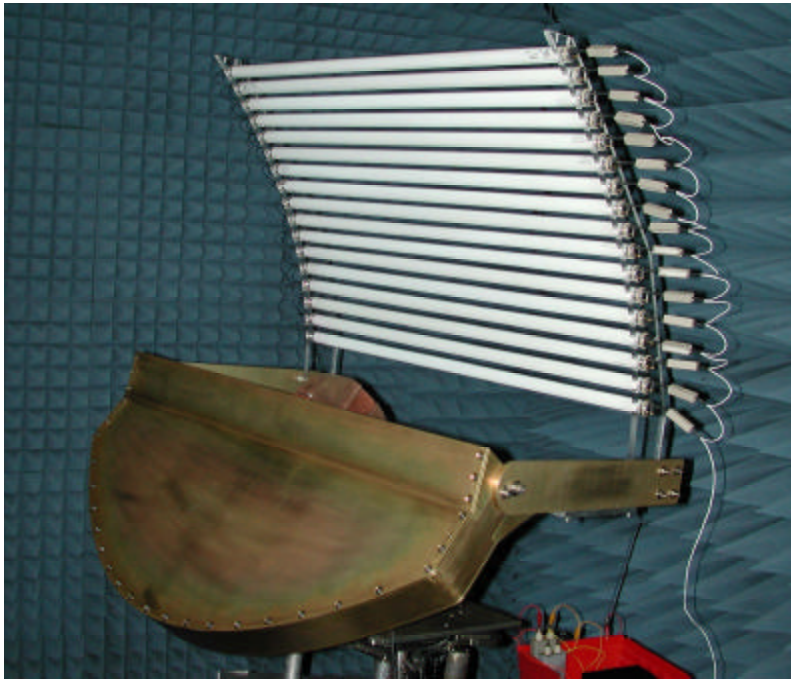
Figure 9: Plasma reflector [From 7].
