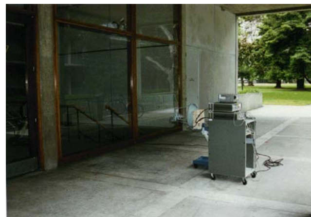
Measurement of propagation through building walls
