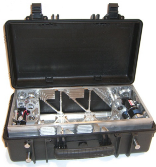
Fig. 6. Layered chassis design. Two latches expose the inside of the robot allowing for easy access for maintenance.
