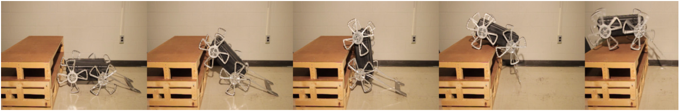
Fig. 9. SeaDog climbing a 48 cm high obstacle. In frame 3, the tail helps to prevent high centering by applying counterclockwise moment to the robot. In frame 4, the tail rotates the robot counterclockwise and acts as a support while the robot is off the ground.
