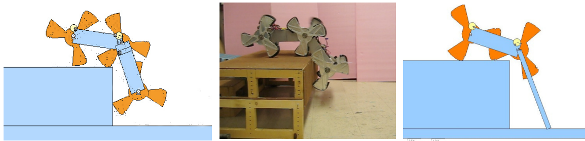
Fig. 5. Screen shot from dynamic simulation of a six wheel-legged Whegs robot with a body joint successfully climbing a 40 cm obstacle; frame from a video of the DAGSI Whegs successfully climbing an obstacle of the same height; dynamic simulation of a four-wheel-legged Whegs robot with a tail climbing a 48 cm obstacle. The middle wheel-leg reaches much further onto the obstacle, even at this greater height, decreasing the chances of high centering.
