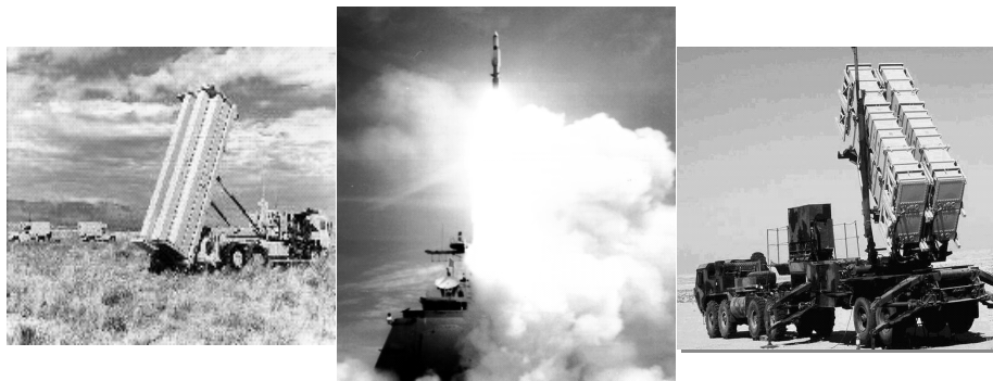
Figure 3. TBMD platforms, deployable or under development. Shown left to right are a THAAD launch vehicle, an AEGIS guided missile cruiser firing a standard missile, and a PATRIOT launch vehicle.
