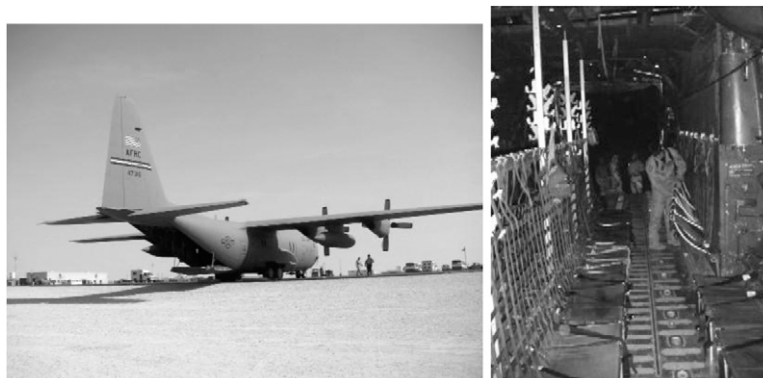
Figure 3. C-130E at Al Udeid. The tail ramp is positioned to transfer cargo pallets by fork lift or roll-on, roll-off k-loader vehicle. The C-130 has a single roller-rail track for manually pushing cargo pallets forward, or aft, or off. For scale, author Dell is standing under the inboard starboard engine. In the image on the right, an aircrew member folds up hammock seats in a configuration change to make room for another cargo pallet.
