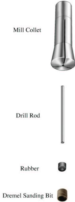
Fig. 3 CNC sanding bit
