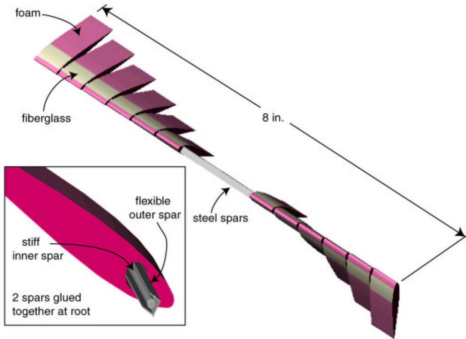
**Fig. 2 The sectioned wing concept**
