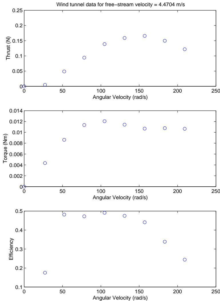
**Fig. 9 Low-speed (4.5 m/s) test results**
