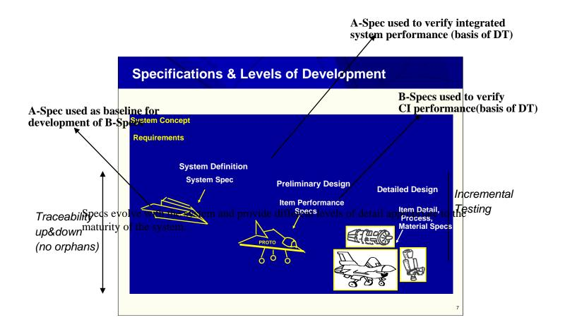
Specs and Levels of Development shows the relationship between the types of specifications and the levels of development of the system. The key point here is that they need to be traceable between levels. In the preliminary design phase when we are developing prototypes, we are also developing "Item Performance", SW or old B Specs for the Configuration Items.
