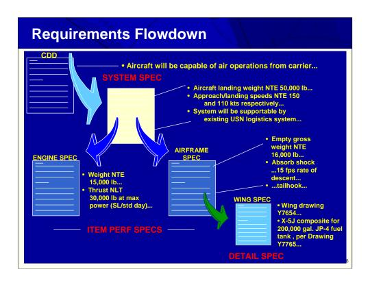
This shows a sample flow-down of the type of information from the CDD to the item detail spec of a typical system.
