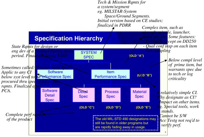
The Specification Hierarchy provides more detail on the types of specifications. Note the change to "name" specs and elimination of the "A, B, C, D, E" and their numbers, i.e., no more B-2, C-1 specs for new programs, although you may still find this convention on existing programs initiated prior to 1994.
