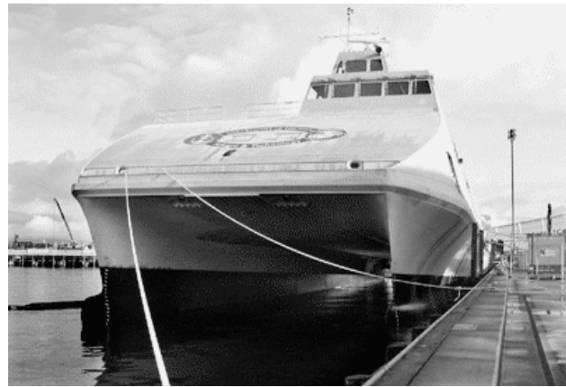
Figure 8: The US Navy experimental ship SEA FIGHTER (FSF1) is 262 feet long, with a beam of 72 feet. Four water jets that are powered by two LM2500 gas-turbine engines or two diesels can drive its 950-ton weight over 50 knots. Source. Department of Defense.
