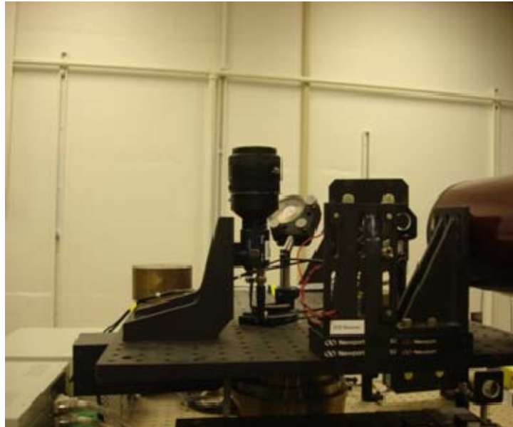
Figure 15. WAT-902H2 SUPREME (EIA) camera used as a star tracker.
