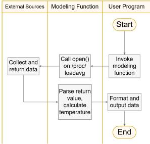
Figure 2. Modified sensors execution flow
