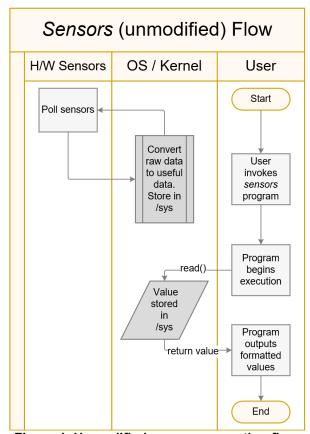
Figure 1. Unmodified sensors execution flow
