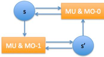
Fig. 12. 1-bit memory brick to remember last selection
