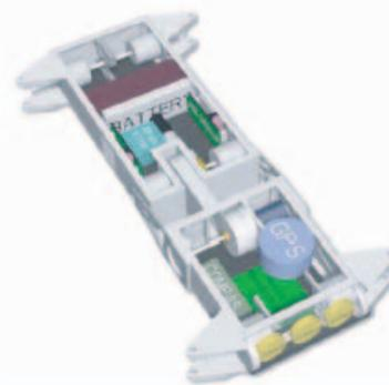
Fig. 12. Another innovation in Whegs<sup>TM</sup> IV is a clear acrylic front panel. This makes it possible to mount infrared sensors or a video camera internally in an area directly adjacent to the main electronics compartment. The rounded shape of the front Panel will have good hydrodynamic characteristics and will also allow it to push up and over irregularly shaped obstacles
