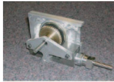
Fig. 11. Whegs<sup>TM</sup> III body joint drive shaft (right) and middle axle (left) in coaxial arrangement
