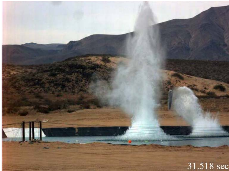
Figure 27. UTT-2(2) get airborne after penetrating the pond bottom [From Boeing 2009b]
