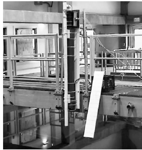
Figure 12. Pneumatic launcher mounted on bridge
