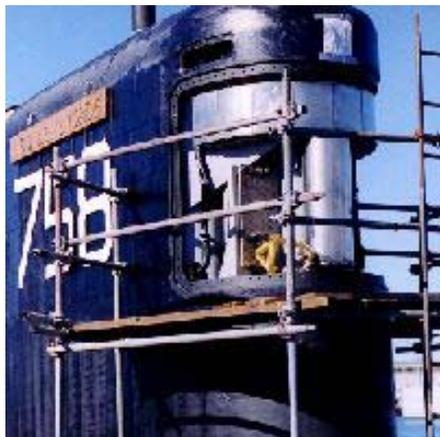
Fig. 2. HF active sonar array mounted in the sail of the USS Asheville, a 688i Los Angeles Class submarine (From N77, 2002).
