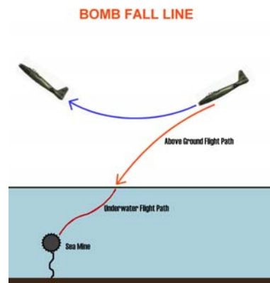
Fig. 1. The concept of airborne sea mine/maritime IED clearance.
