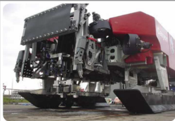
Nautilus has investigated the use of proven subsea technology for mining the SMS deposits. This 900HP ROV oil/gas pipeline trenching machine is as powerful as a D11 bulldozer.
