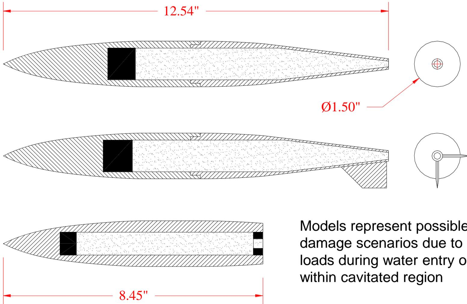
Models represent possible different damage scenarios due to excessive loads during water entry or tail slap within cavitated region
