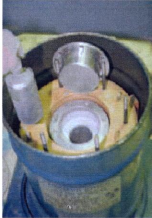
Primary source container being placed into a double-walled secondary container. The inner wall is depleted uranium and the outer wall is stainless steel.
