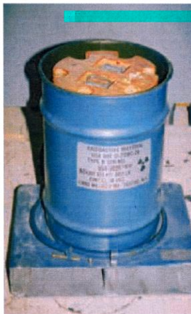
Steel drum outer shipping container with top plywood structure in place.
