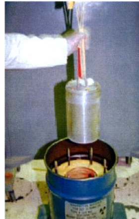
Secondary container being placed into the outer shipping container. The secondary container will be surrounded by laminated plywood in the outer container.
