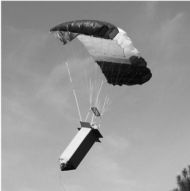
Fig. 2 Test system with deployed parafoil.
