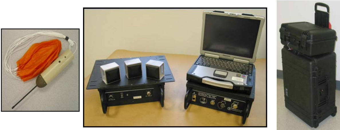
Figure 2. JPADS-MP Fly-Away Kit From Right to Left: Dropsonde, JPADS-MP HW & Laptop & Carrying Case
