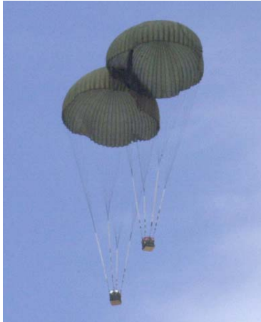
Figure 13. Two AGAS 2000 Flying the Same Planned Trajectory Come Into Contact.
