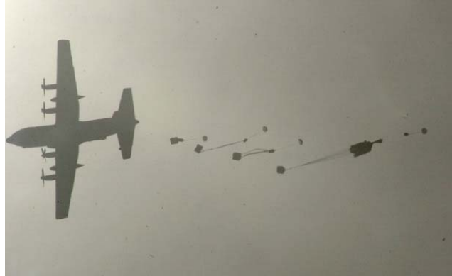
Figure 8. Four AGAS 2000 Deployed from a C-130 Hercules.
