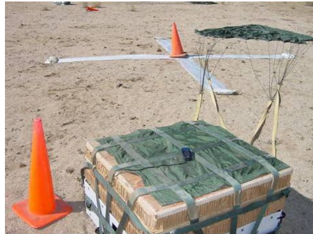
Figure 16. Prototype AGAS 500's T-10R Covers Target IP in Development Test.
