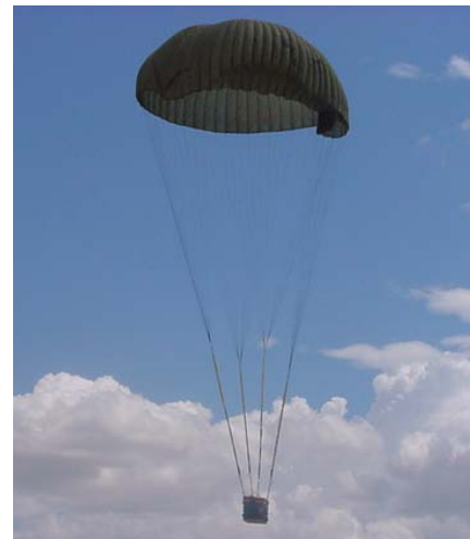
Figure 2. AGAS 2000 in a Commanded Riser Slip.
