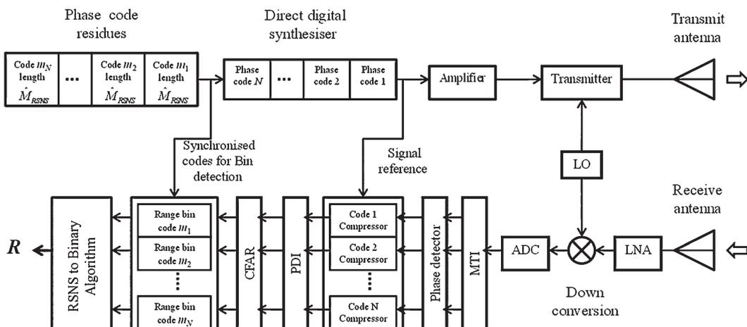
**Fig. 4** Block diagram for the radar using  $N$  residue-P4 phase code sequences
