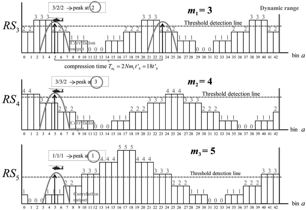
Fig. 7 Illustration of target detection by using the range bin matrix for RSNS-P4 code with  $m_1 = 3$ ,  $m_2 = 4$  and  $m_3 = 5$
