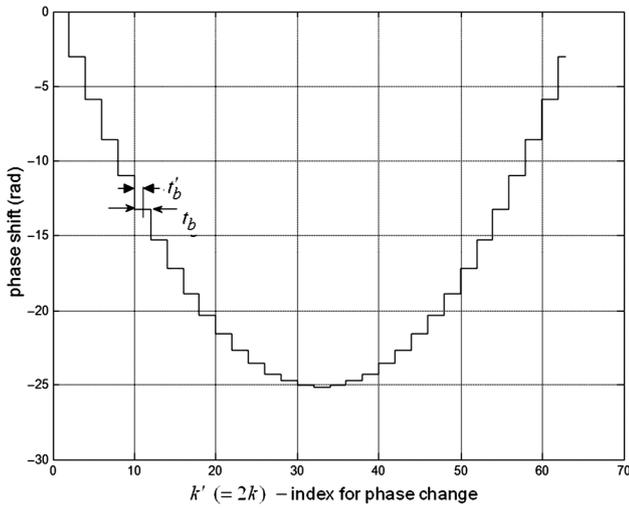
**Fig. 3** Symmetrical residue-P4 subcode phase values within a code period using  $m_1 = 16$ ,  $N = 2$  and  $N_{c_1 \text{ RSNS}} = 64$  shown with the P4 subcode phase values using  $N_{c_1} = 32$
