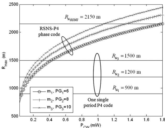
Fig. 8 Comparison of the maximum unambiguous range of CW radar system for  $SNR_{R_{out}} = 13$  dB using the RSNS-P4 code for  $m_1 = 3$ ,  $m_2 = 4$  and  $m_3 = 5$  against using each P4 code individually for  $N_{ci} = N_{ci_{RSNS}}/N$
