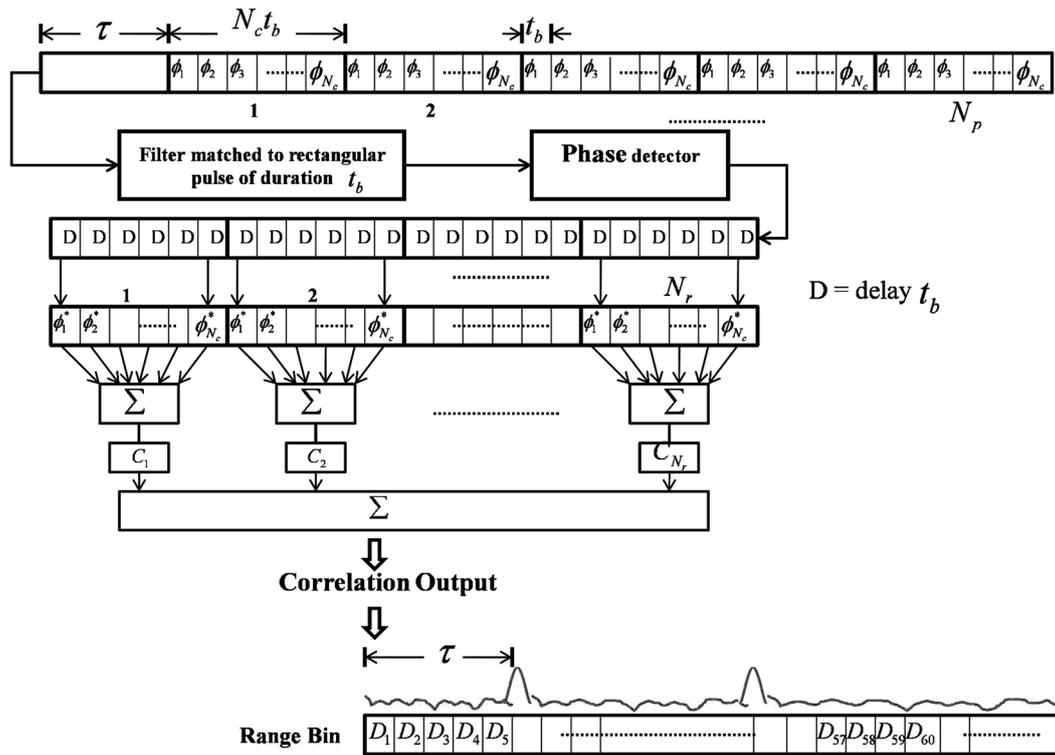
**Fig. 1** Compression receiver matched to  $N_r$  periods of a transmitted polyphase code for  $v = 0$  and the receiver's range bin for detection (adapted from [2])
