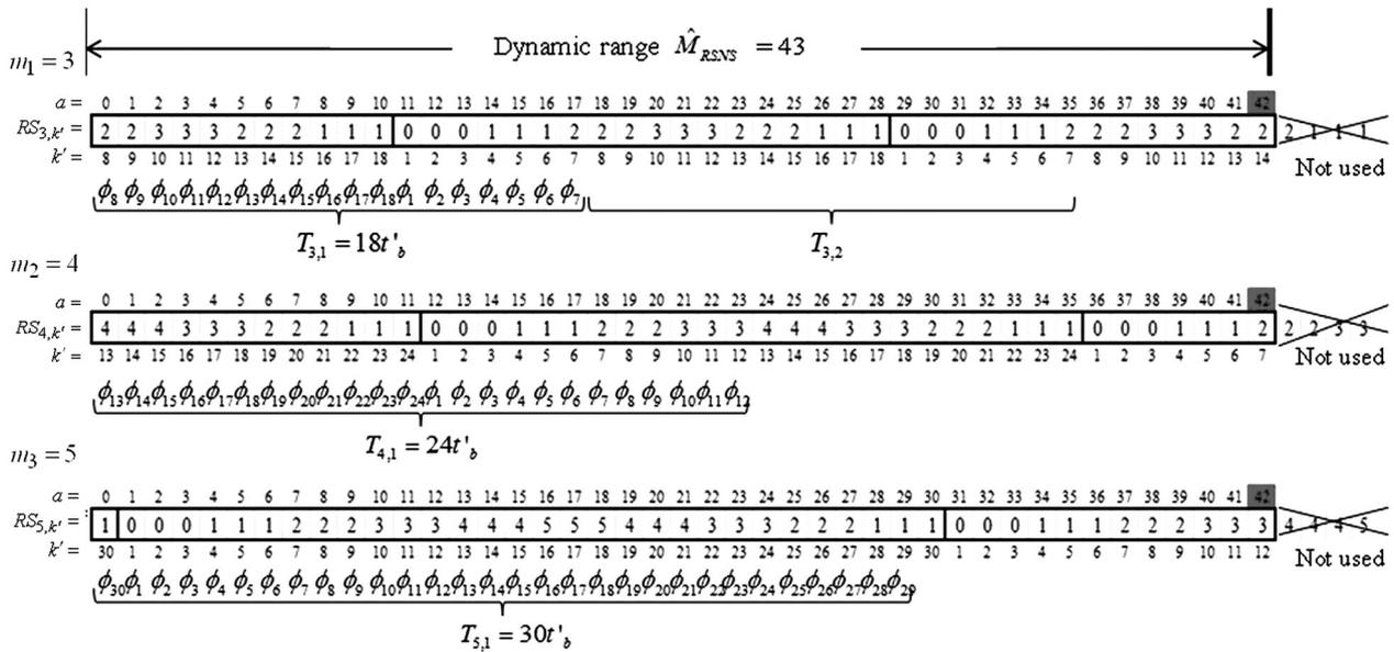
Fig. 5 Illustration of transmitted signal using  $N = 3$  robust symmetrical residue-P4 phase code sequences for  $m_1 = 3$ ,  $m_2 = 4$  and  $m_3 = 5$
