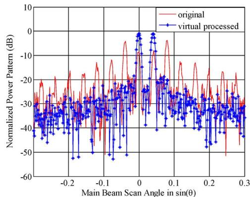
Fig. 6. Comparison of original and synthesized antenna response after virtual filling for an element level SNR of 6 dB with 20 dB sidelobe tapering.
