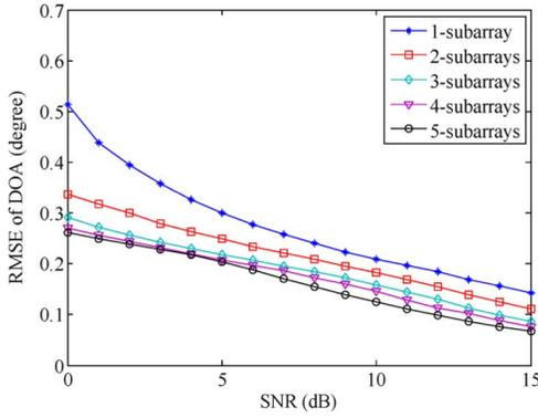
Fig. 4. RMSE of DOA for signal 2 versus SNR per element for various numbers of subarrays. Each subarray has 80 elements spaced  $0.42\lambda$ , and gaps are equal to the subarray size.
