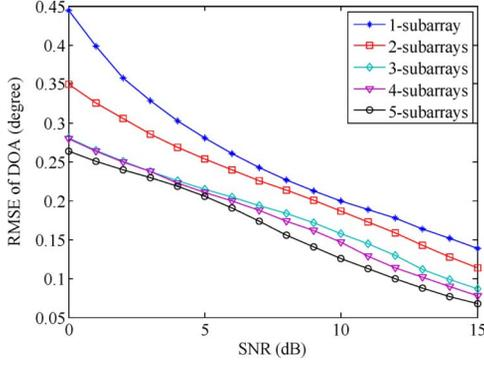
Fig. 3. RMSE of DOA for signal 1 versus SNR per element for various numbers of subarrays. Each subarray has 80 elements spaced  $0.42\lambda$ , and gaps are equal to the subarray size.
