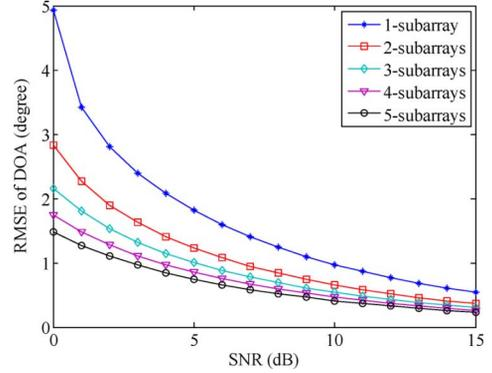
Fig. 2. RMSE of DOA for one signal versus SNR per element for various numbers of subarrays. Each subarray has eight elements spaced  $0.42\lambda$ , and gaps are equal to the subarray size.
