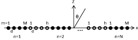
Fig. 1. Linear distributed digital subarray model. Black filled dots are real elements, and nonfilled dots are virtual elements.
