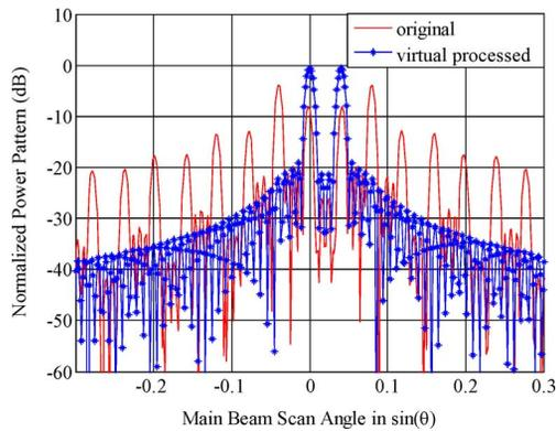
Fig. 5. Comparison of original and synthesized antenna responses of five subarrays each with 30 elements, for signals of equal power (noiseless) incident from  $0^\circ$  and  $2.3^\circ$ .
