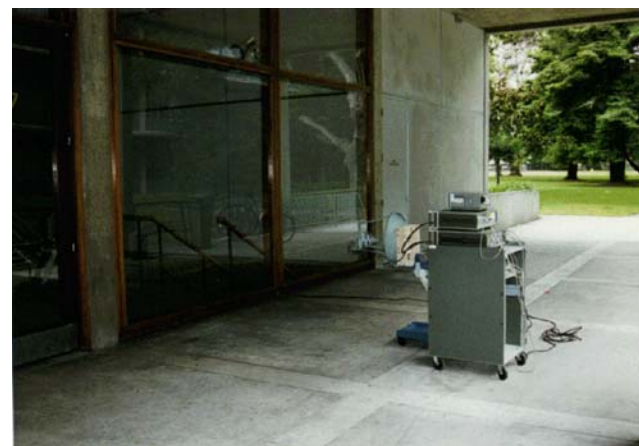
Measurement of propagation through building walls
