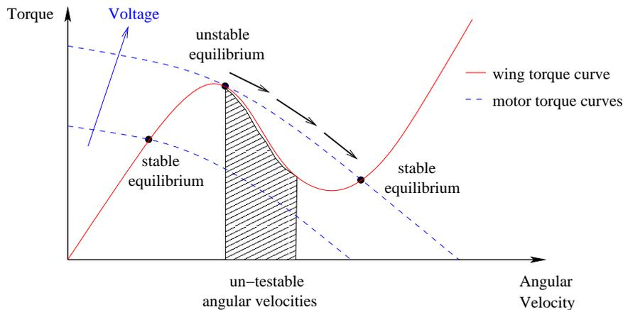
Fig. 11 Motor and wing torque curves effect on twist angle instability
