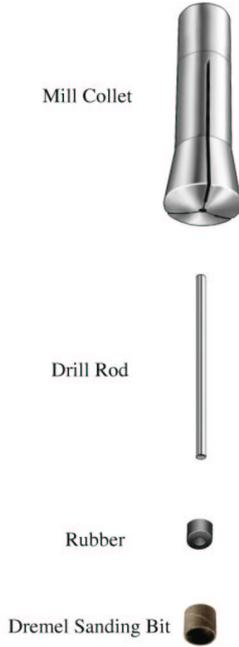
**Fig. 3 CNC sanding bit**
