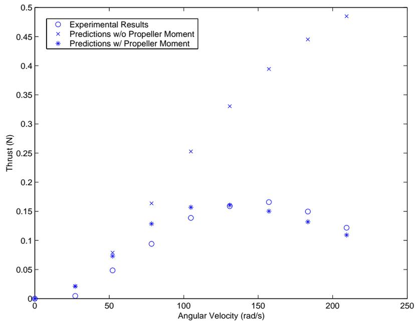
**Fig. 8 Comparison of experiment with model including propeller moment**
