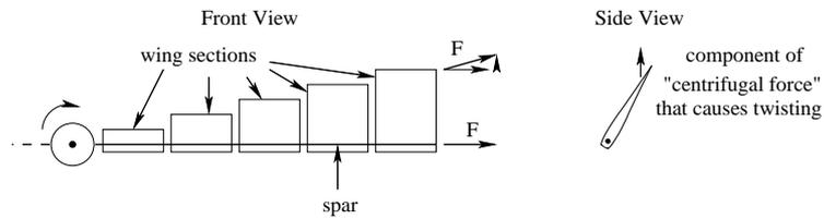
**Fig. 7 "Centrifugal force" view of propeller moment**
