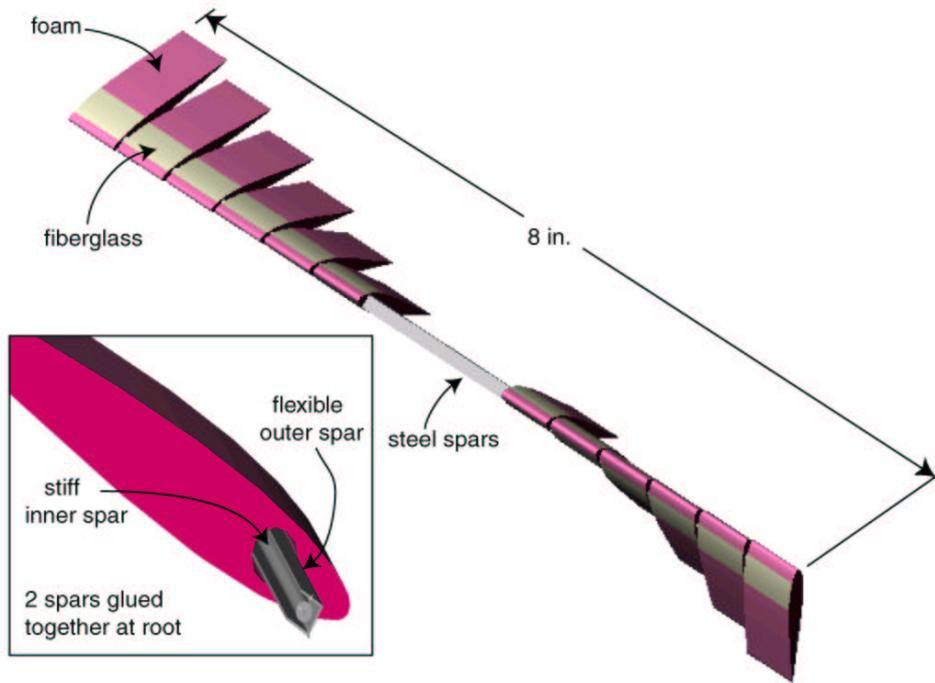
**Fig. 2 The sectioned wing concept**
