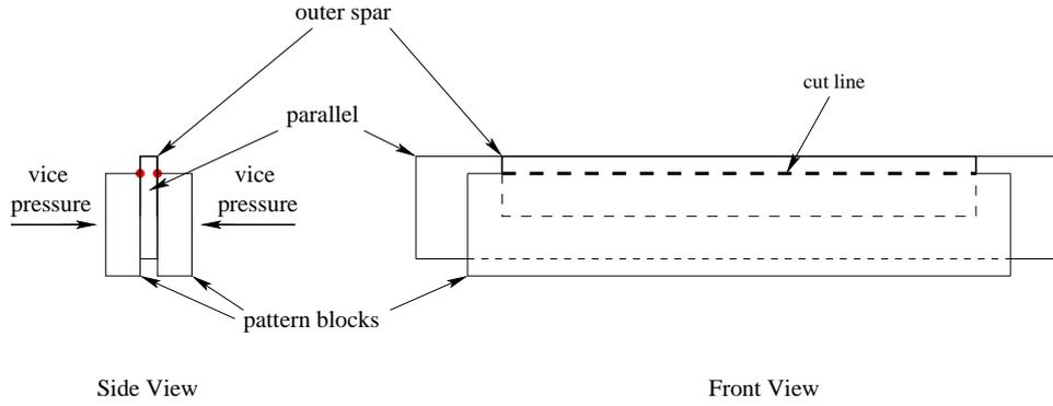
**Fig. 4 Spar trimming technique**
