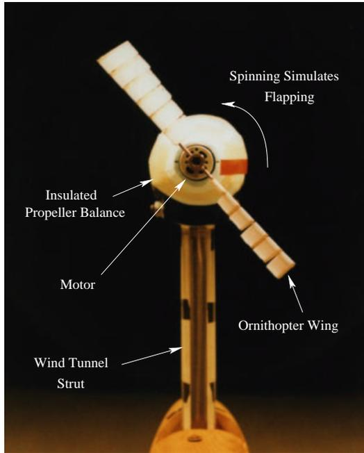
**Fig. 1 Ornithopter wing fitted to propeller balance**
