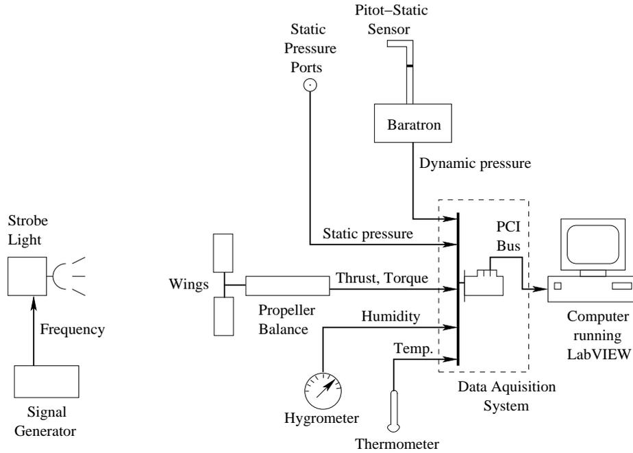
Fig. 5 Schematic of instrumentation used to quantify ornithopter wing performance
