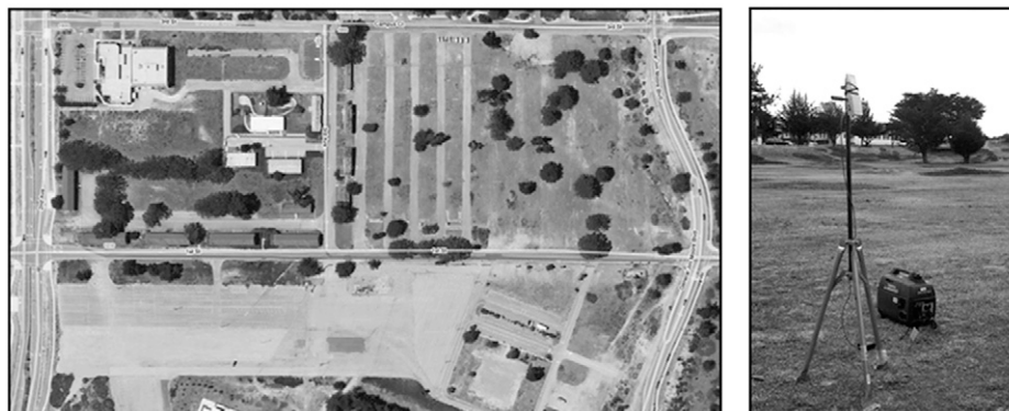
Figure 9. Field testing in Fort Ord, California. Left: Aerial view of 45-acre Fort Ord operating region [image courtesy Google Maps ( http://maps.google.com )]. Right: Wireless mesh access point, mast, and portable generator
