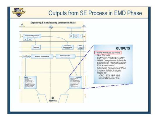
Take a look at the blow-up of the Outputs block from the Systems Engineering Process in the Engineering and Manufacturing Development phase. Most of what's there is very similar to the Output block of the SE Process in the Technology Development phase. One of the things that *is* different is the Initial Product Baseline.
