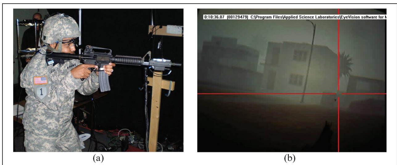
**Figure 11.** (a) A soldier engages targets in the virtual environment. The weapon is an M4 carbine mounted with an interactive laser, and the soldier wears the Mobile Eye system. (b) The video image captured by the eye-tracking system.
