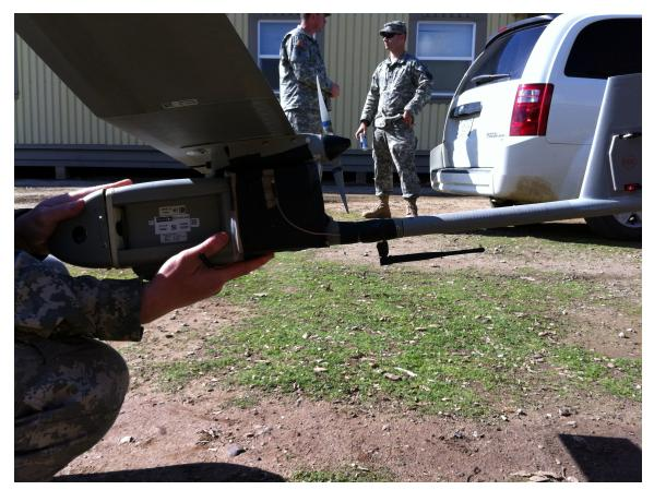
(Enclosure 2) Wave Relay Single Board Module Mounted on Raven 11B
