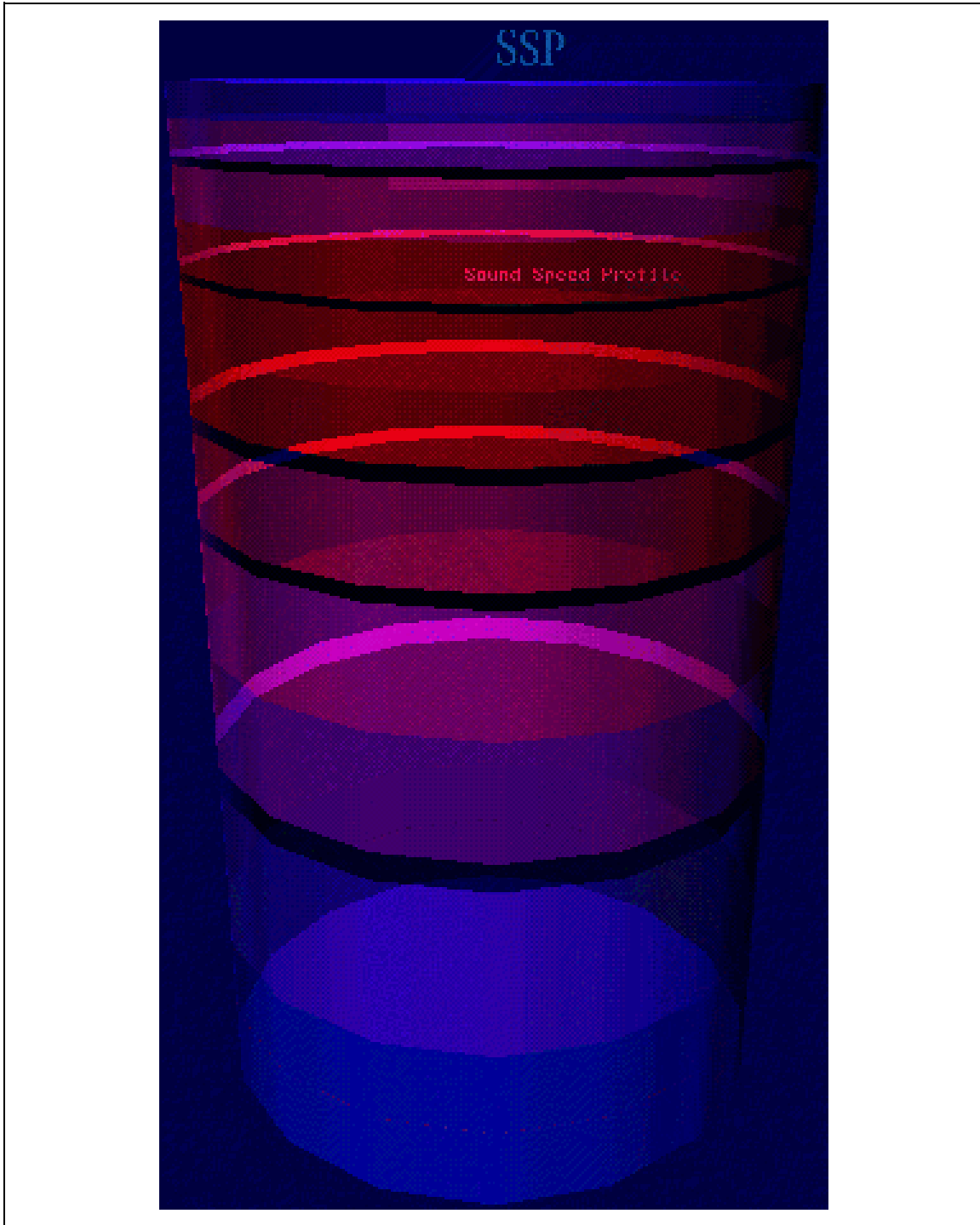
Figure 8.6. Example graphics visualization of subsampled Sound Speed Profile (SSP). Sound speed is mapped to cylinder color at intervals proportional to local depth, producing a 3D information icon.
