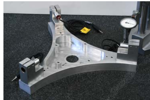
Figure 14. Inspection of laser source assembly on granite table with precision height meter.
