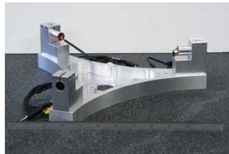
Figure 7. Laser source subsystem, including diode lasers, mounts, and top boomerang.
