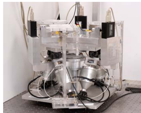
Figure 3. NPS Hexapod with the laser metrology system.
