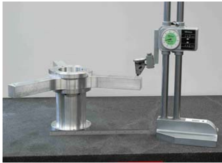
Figure 13. Inspection of base cylinder and bottom boomerang on granite table with precision height meter.
