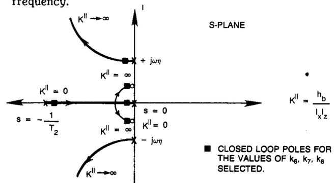
**Figure 5: ROOT LOCUS FOR TYPE (c) TRANSITION CONTROLLER**
