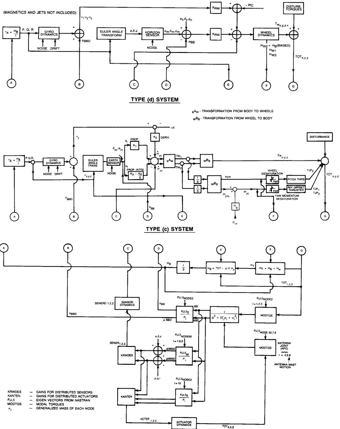
Figure 6: NONLINEAR SIMULATION MODELS (Types (a) & (b) are similar to Type (d))
