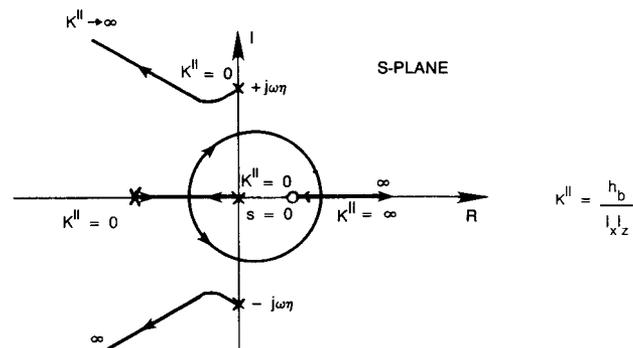
**Figure 4: ROOT LOCUS FOR TYPE (c) NORMAL MODE CONTROLLER**
