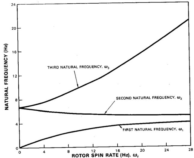
FIGURE 2. NATURAL FREQUENCIES FOR DUAL-SPIN STABILIZED SPACECRAFT
