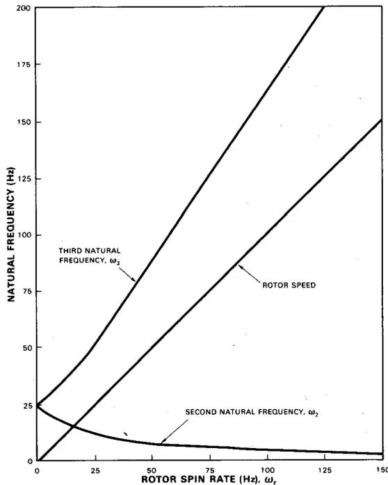
FIGURE 4. NATURAL FREQUENCIES OF BODY-STABILIZED SPACECRAFT
