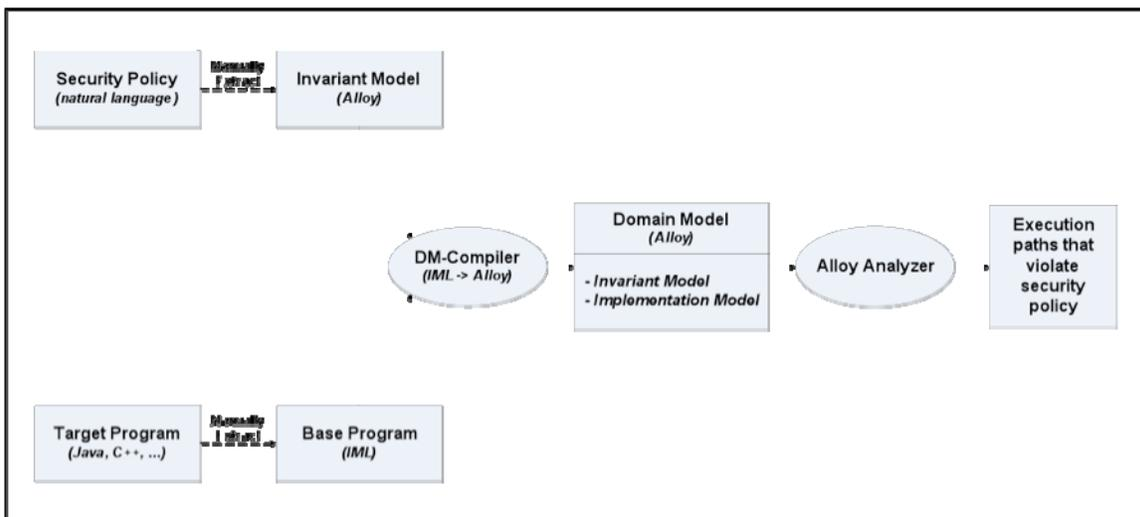
Figure 1. Domain Model approach to system security verification.
